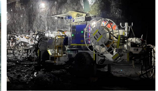
Electric underground drill rigs
