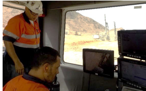
Remote blast hole drilling
