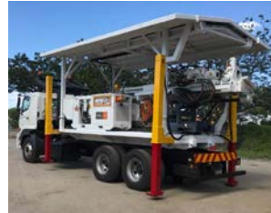
In pit horizontal diamond drilling / De-watering
